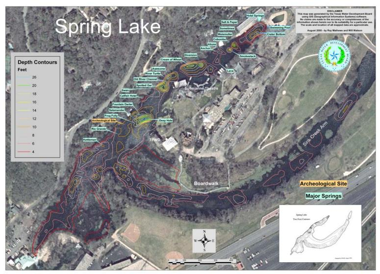
Figure 1. GPS-DOQ map of Spring Lake. Major springs and habitat features are shown with depth contours; based on hydrographic survey, depth and GPS measurements.
