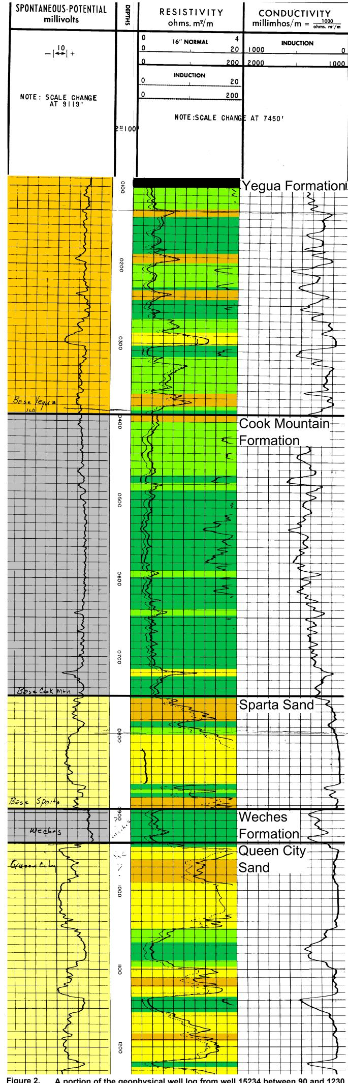
A portion of the geophysical well log from well 15234 between 90 and 1230 feet below ground surface. The left track of the log shows the Spontaneous Potential curve with superimposed estimated salinity class The center track shows depth below ground surface in units of feet. The right track shows the shallow and deep resistivity curves (solid and dashed lines, respectively) with superimposed lithology interpretations The far right track shows the induction conductivity curve.
