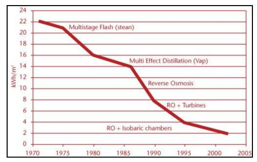
Figure 1-Evolution of energy consumption for the desalination of seawater over the last 30 years (authors estimation based on historical records). Note 1k m3/hr = 6.3 mgd; 75 bar = 1,090 psi
