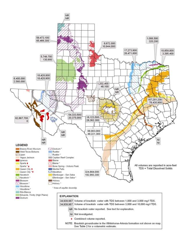
Figure 4 Volumetric estimates of brackish groundwater in the minor aquifers of Texas (data modified from LBG-Guyton Associates, 2003)
