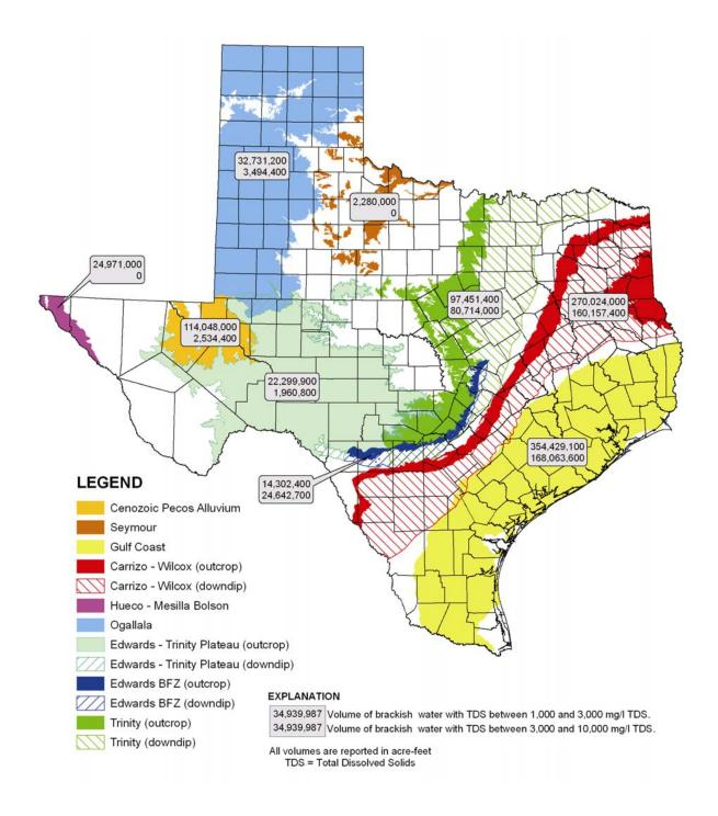
Figure 3 Volumetric estimates of brackish groundwater in the major aquifers of Texas (data modified from LBG-Guyton Associates, 2003)
