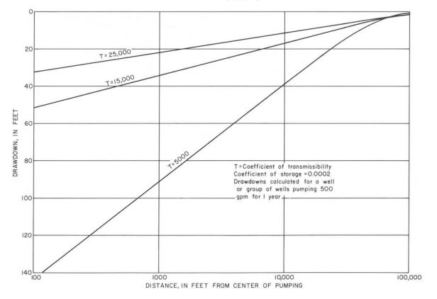
Figure 7.-Relation of Drawdown to Distance for Various Coefficients of Transmissibility
