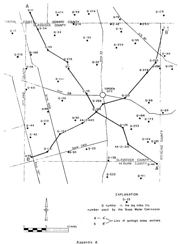
Location of Wells Used for Subsurface Control and Geologic Cross Sections
