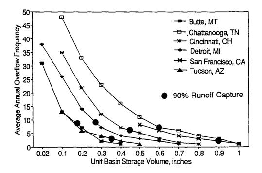
Figure 2b: Basin Overflow Frequency Versus Unit Storage Volume
