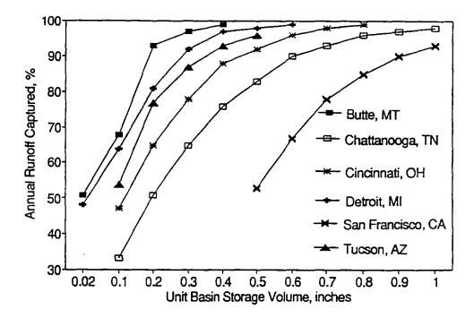
Figure 2a: Runoff Capture Efficiency Versus Unit Storage Volume
