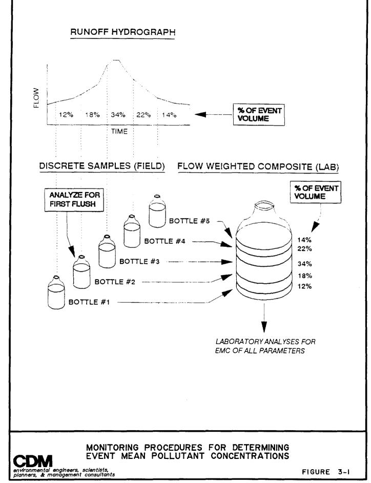
mark on the flow strip chart each time a sample is collected. After a storm event, the flow strip chart can be analyzed to select those samples that best represent the storm hydrograph. Selected samples would be manually composited after the storm to produce a single flow-composite sample.
