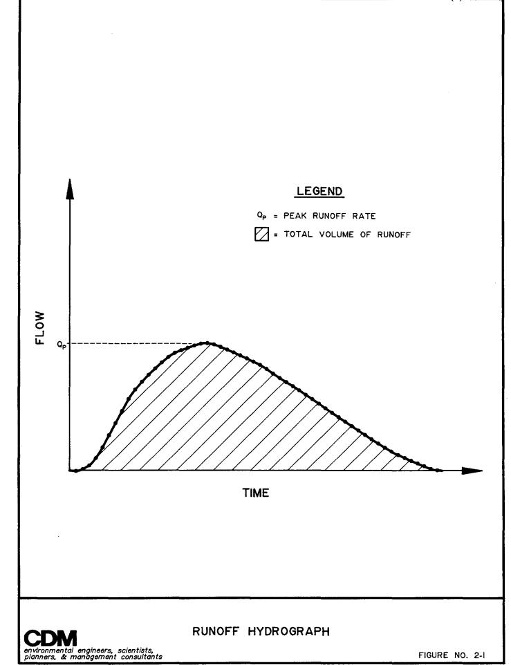
to determine the total volume of runoff for a given storm. Therefore, the Rational Method is inappropriate for use in water quality modeling efforts since total annual or seasonal runoff quantities would be required.
