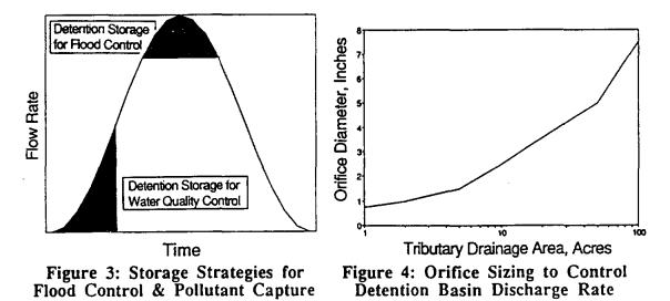
Caution should be exercised when retrofitting the small outlet control conduit for water-quality detention in an existing flood-control detention facility. In particular, the flood control performance of the basin must be evaluated for larger
