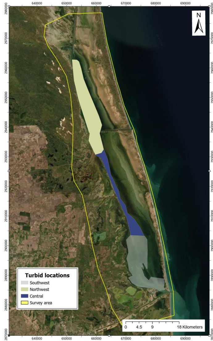
Figure 22: Sections of Lower Laguna Madre with higher turbidity concentration in May 2017. These sections were suggested for sonar mapping to build a complete hydrographic mapping of the lagoon.
