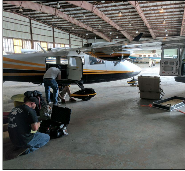
Figure 17 (b): BEG researchers are installing the AHAB Chiroptera Lidar system and other required equipment in the Partenavia P68-C aircraft.
