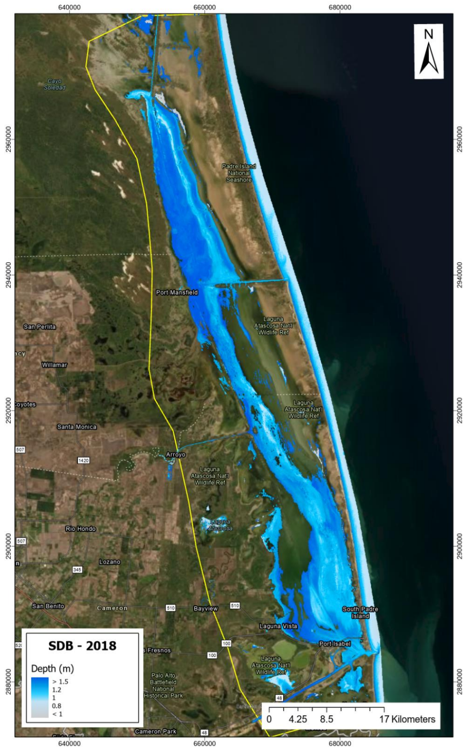
Figure D-3: SDB of Laguna Madre as derived from 17/05/2018 Sentinel-2A L1C imagery. Analysis indicated 1.71 m as the deepest, and depth range was 2.24 m.
