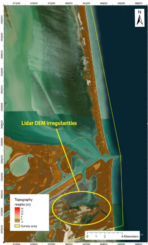
Figure 39: Visible NIR Lidar irregularities caused by the classification algorithm. Height interpolation and averaging method with neighbouring distance parameters were used to fill some of these void areas.
