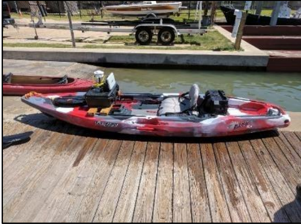
Figure 11 (a): In-situ measurements in Lower Laguna Madre. BEG measured depths using a single-beam Garmin sonar installed onto a kayak.
