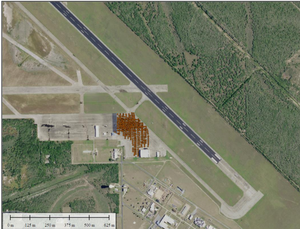
Figure 7: The red dots illustrate 446 GPS survey points acquired using a Trimble R8 GNSS receiver in the taxiway of Port Isabel-Cameron County. Positional measurements were refined by post-processing method using the TxDOT maintained TXLN GPS base station.
