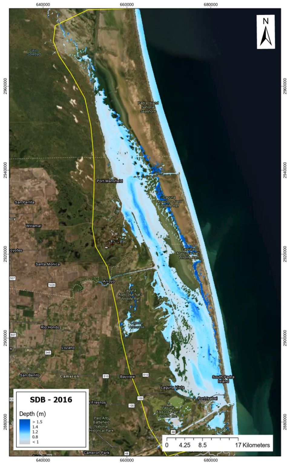
Figure D-1: SDB of Laguna Madre as derived from 05/12/2016 Sentinel-2A L1C imagery. The deepest location measured was 2.34 m.
