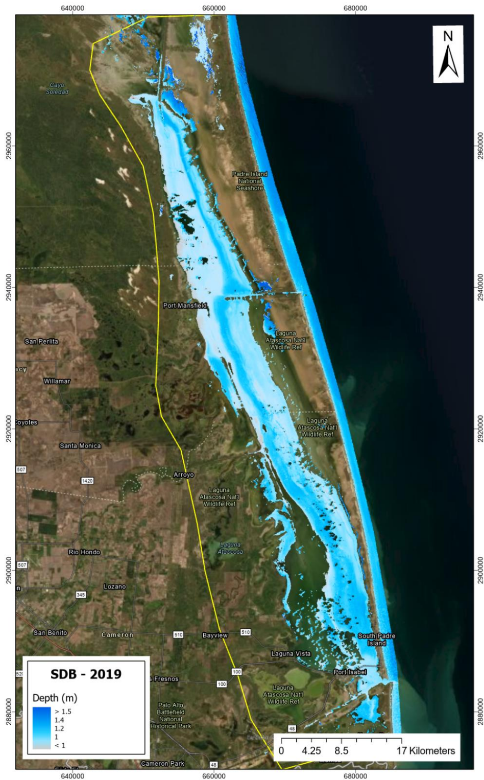
Figure D-4: SDB of Laguna Madre as derived from 27/05/2019 Sentinel-2A L1C imagery. The depth range and the maximum depth was 2.54 m.
