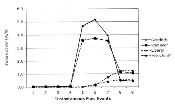
Figure 9. Stream power at Trinity River gaging stations for nine Hurricane Rita instantaneous flows, based on discharge and upstream (import) or downstream (export) slope.
