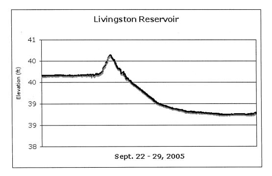
Figure 4. Water surface elevations for Lake Livingston for the week including Hurricane Rita, showing the rise in lake levels and subsequent drawdown via dam releases to assess and repair damages.
