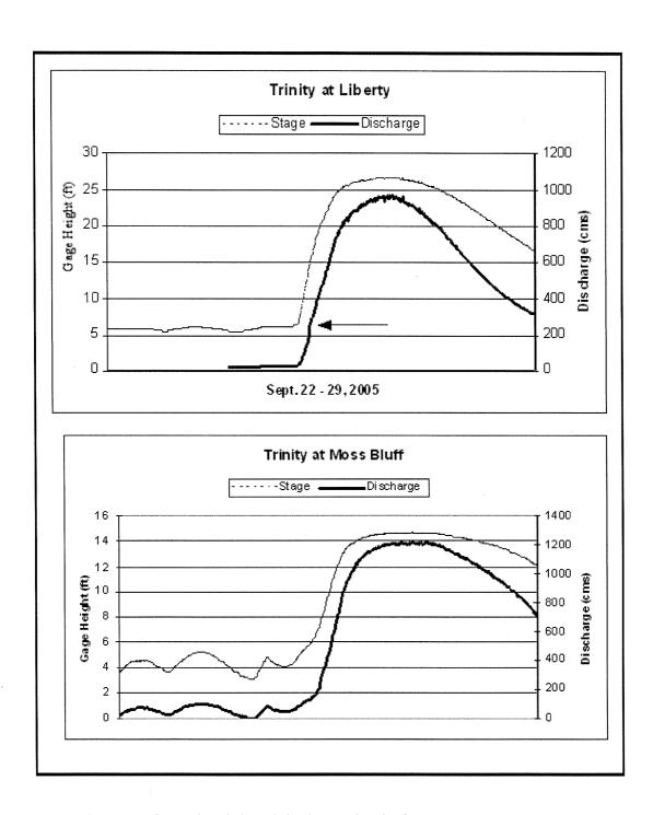
Figure 6. Stage (gage height) and discharge for the lower Trinity River at the Liberty and Moss Bluff gaging stations, with readings every 15 minutes. For the Liberty data, discharge was estimated by the author for the portion of the curve prior to the point indicated by the arrow. For Moss Bluff, discharge is entirely estimated by the author.
