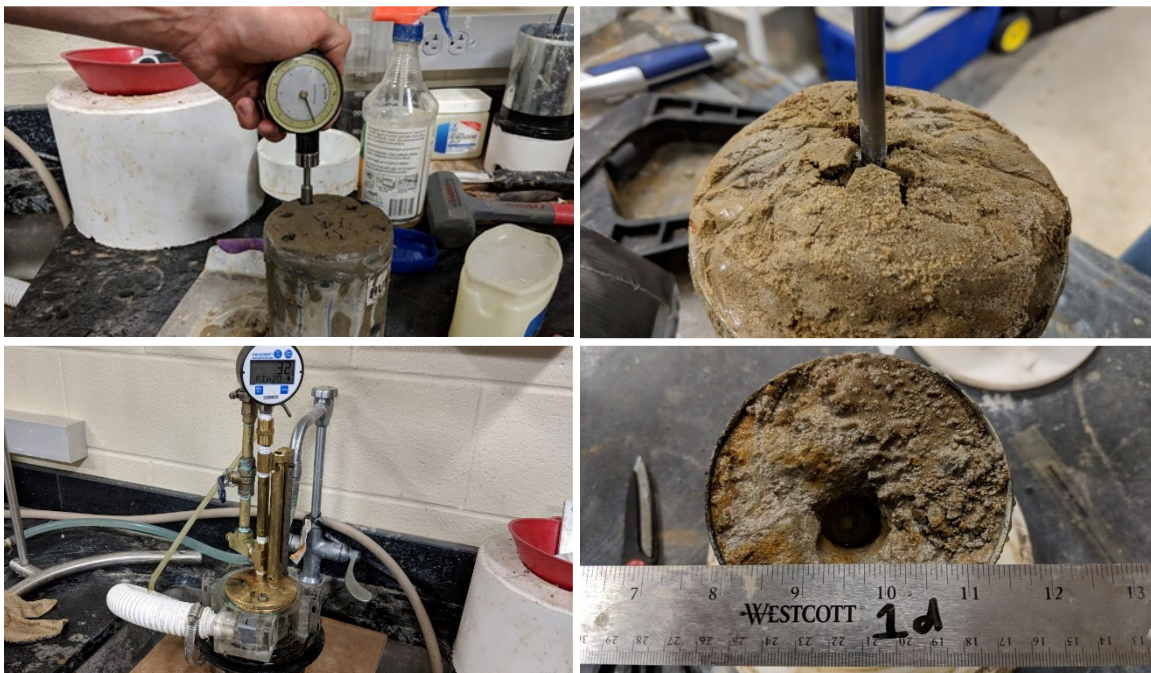
Figure 2-23. Photographs showing laboratory processing of core samples using (clockwise from upper left) a penetrometer, vane, jet pressure tester, and a post-jet testing core.
