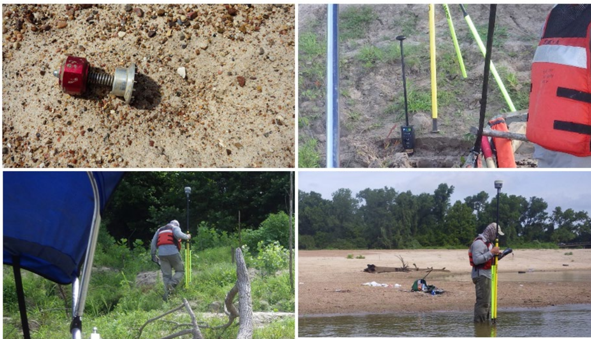
Figure 2-22. Photographs showing (from left to right) field vane, hydrometer, bank RTK GPS surveying, and channel RTK GPS surveying.
