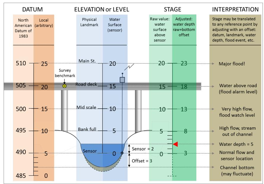
**Hypothetical stream cross-section, bridge, and sensor with stage interpretations.** Water depth is determined from raw sensor value (2) + bottom offset (3) = 5.
