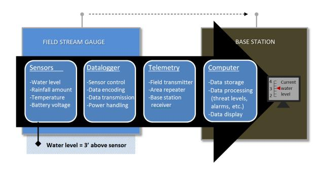
Figure 3.2 Data flow from field stream gauge network to base station at receiving center
