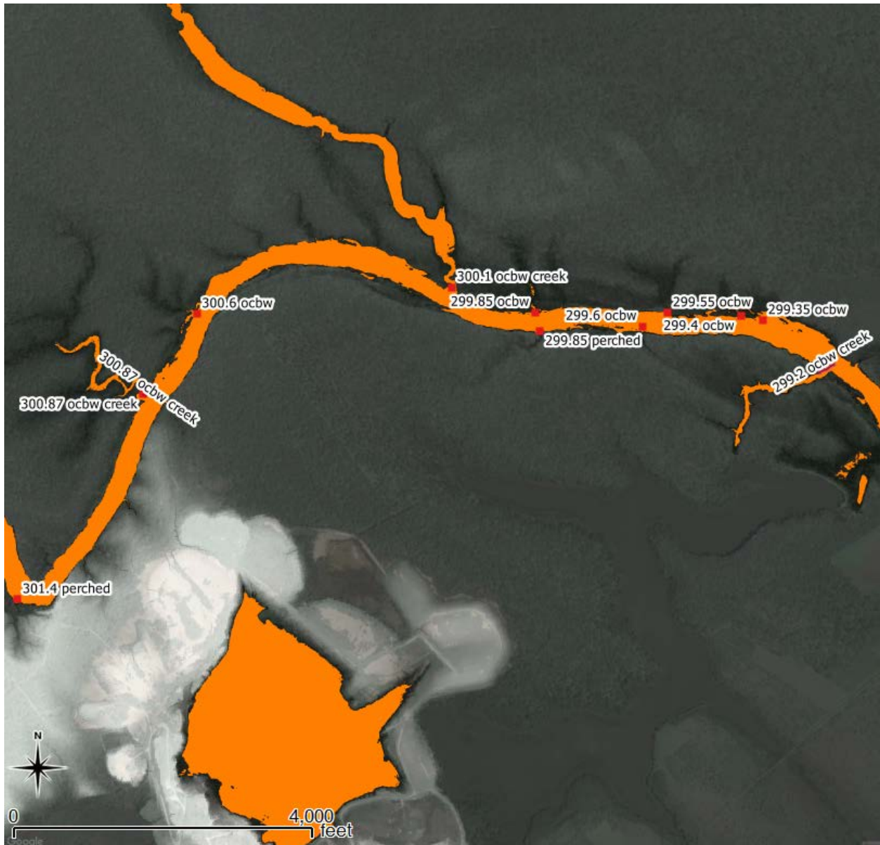
Figure 27. Segment C3 upstream of 080295 1 of 4- Observed inundation and connectivity areas over the RAS 13400cfs inundation map (orange). Note: Numbers represent approximate river mile.
