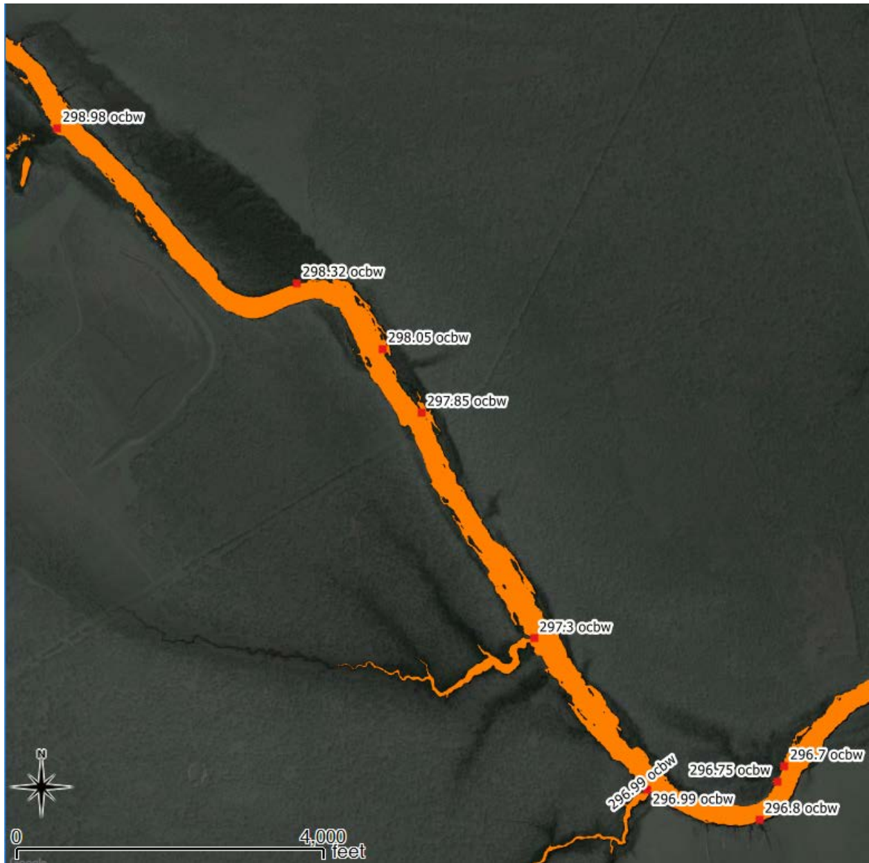
Figure 28. Segment C3 upstream of 080295 2 of 4 - Observed inundation and connectivity areas over the RAS 13400cfs inundation map (orange). Note: Numbers represent approximate river mile.
