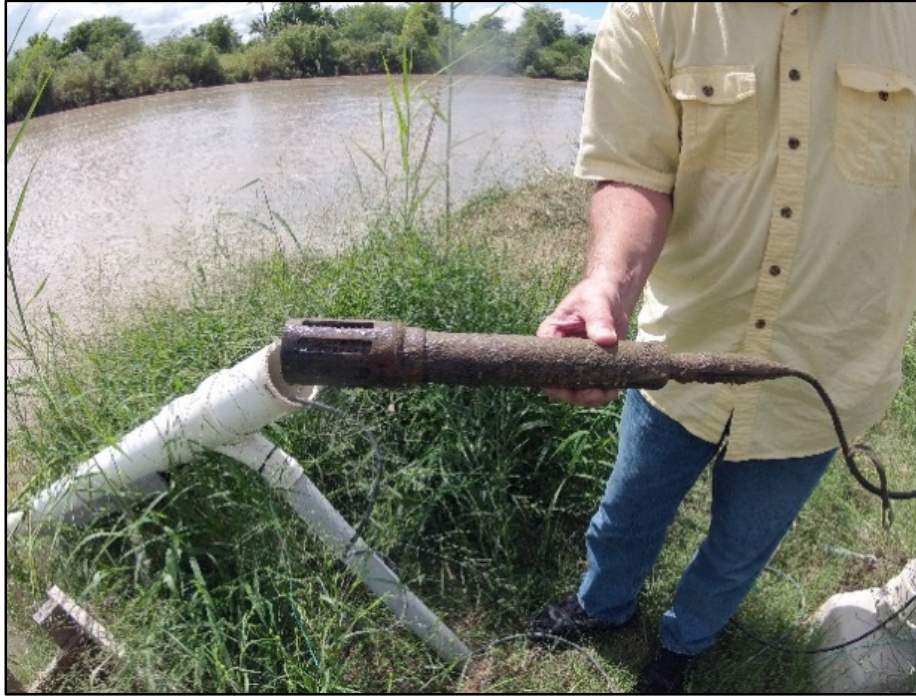
Figure 7. CAMS 789. YSI water quality meter immediately after retrieval from the river. Photo by Freese and Nichols, Inc. September 29, 2014.
