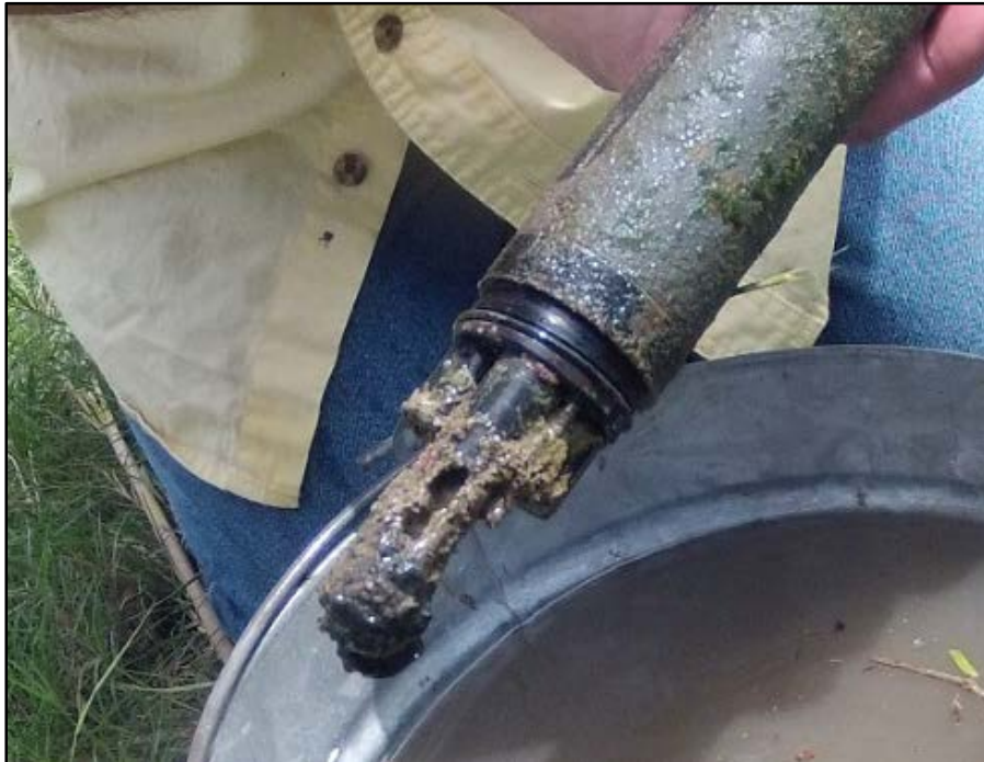
Figure 8. CAMS 789. YSI water quality meter with fouling on probes. Photo by Freese and Nichols, Inc. September 29, 2014.
