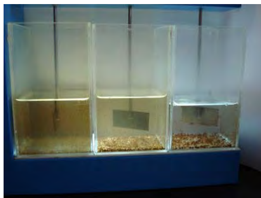
Exhibit 3-1 Coagulation Effects in Jar Testing
