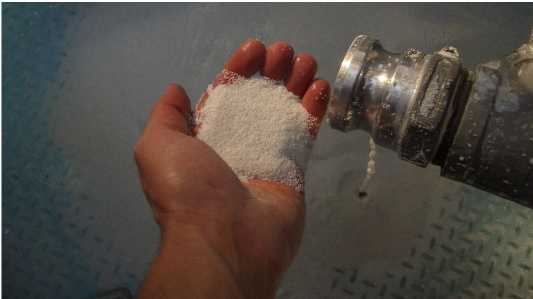
Figure 3-15. Calcite pellets from the intermediate pellet softening process.
