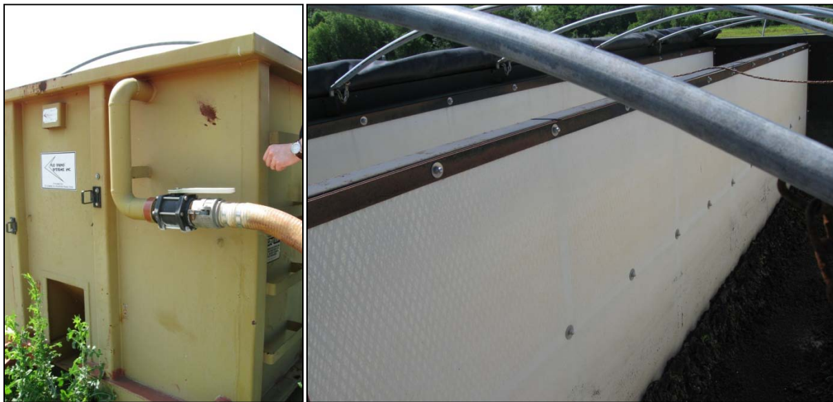
Figure 1.14 Solids Dewatering Dumpster at the City of Van Alstyne
