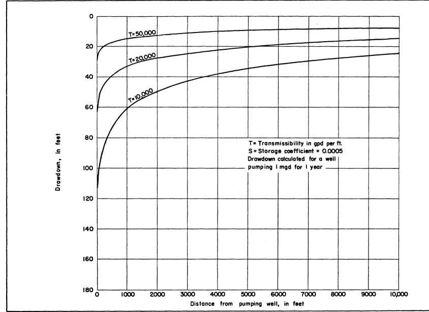
FIGURE 5. - Relation between drawdown and transmissibility in an infinite aquifer
