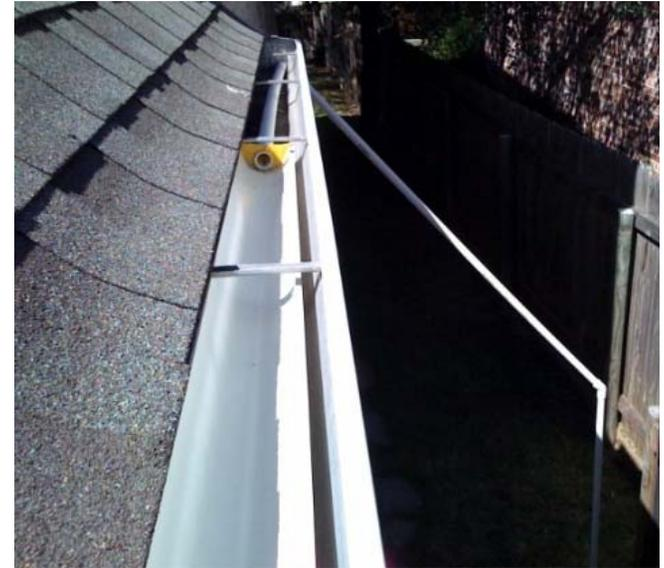
Sampler gutter insert.
