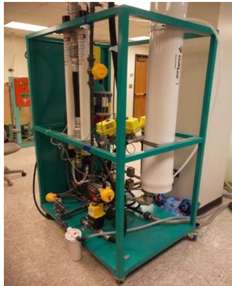
Figure 2-3. Pilot RO system membrane housing pressure vessels and holding tank.
