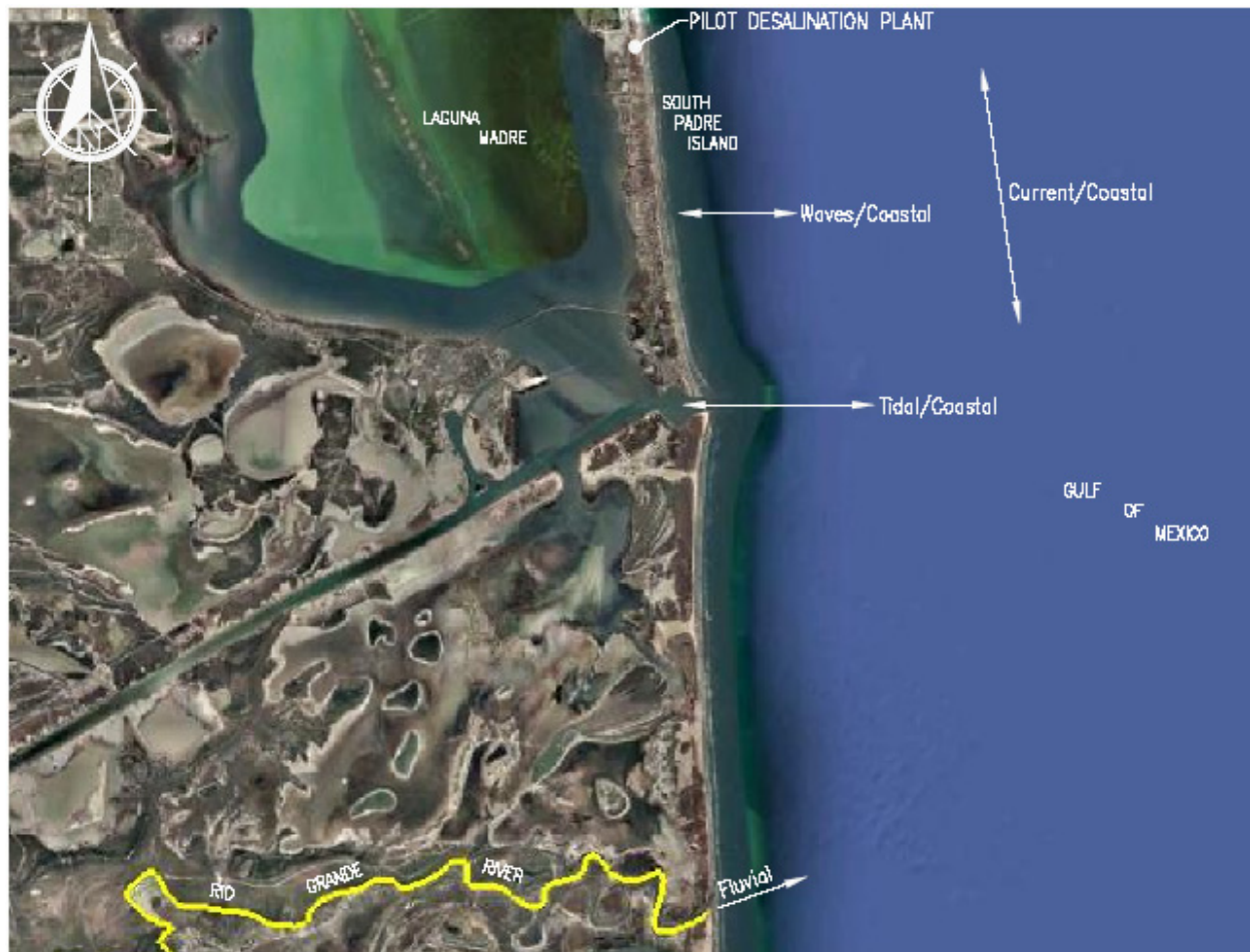
Figure II-35: Sediment transport in pilot vicinity.
