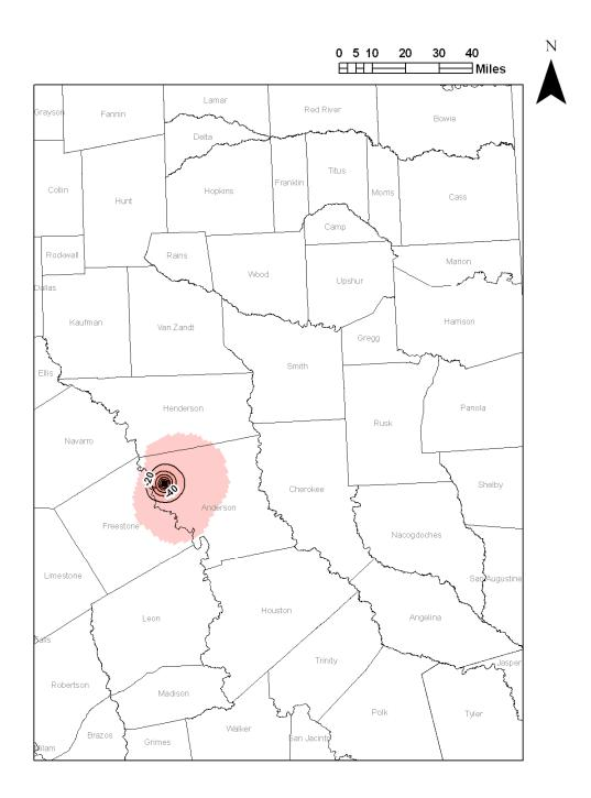
Figure 2. Water level declines in the Middle Wilcox Aquifer after four years of pumping compared with pumping only baseline 1999 amounts. Shaded area represents declines greater than one foot and contour interval is 20 feet.
