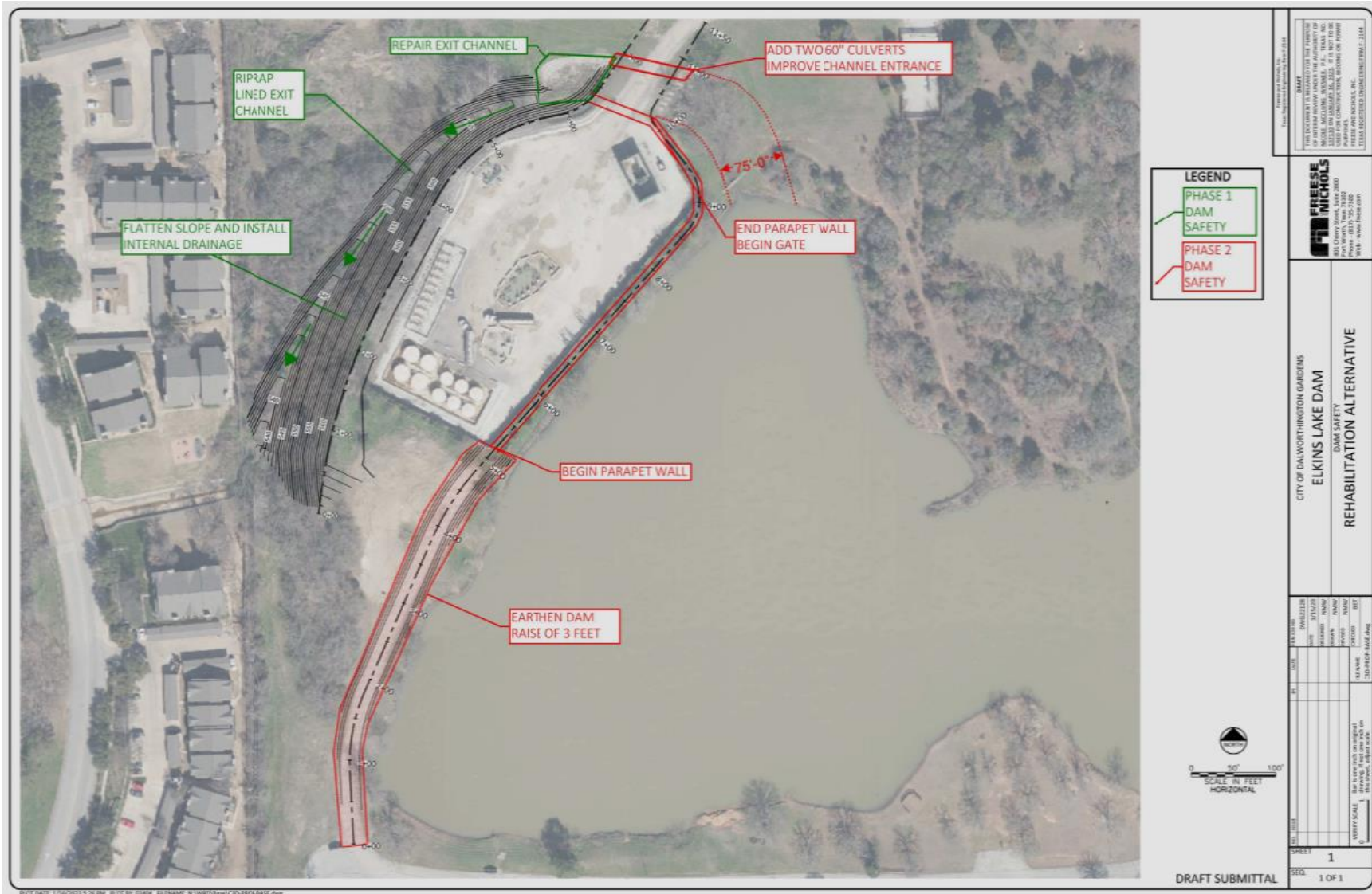
Figure F.31. Elkins Lake Dam Rehabilitation (FMP 033000072)
