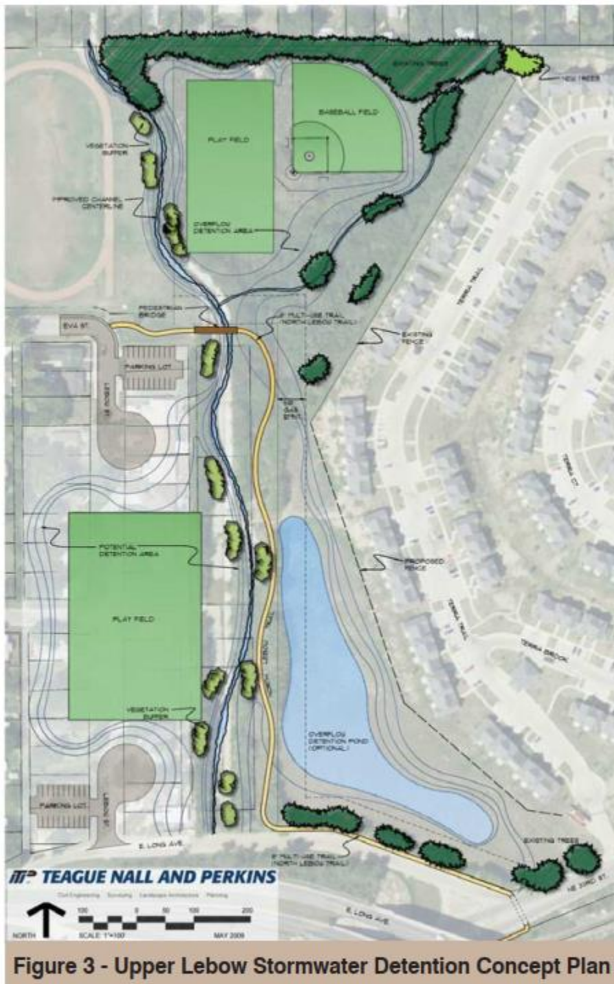
Figure F.34. Upper Lebow Storm Water Detention Facility
