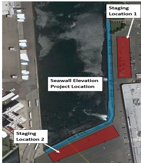
Figure 2. Example of a project site map. Map clearly shows the project area in blue and two staging areas in red. The site features are overlaid on an aerial photo.
