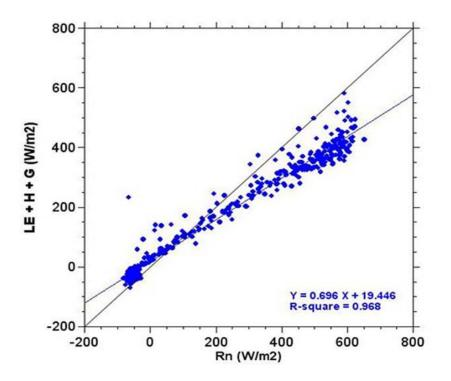
Figure 34. Energy balance closure for Field 15 considering only steady-state terms.
