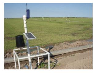
transmitters (950T1) sending wireless soil moisture data to a receiver (950R1data logger), powered by a solar panel, and connected to a rain gage. Water meter attached to the sand-media filter, located downstream from the pivot.
