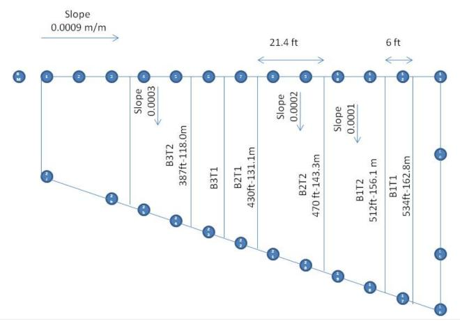
Figure 1 Field experiment setup for two treatments and 3 repetitions.
