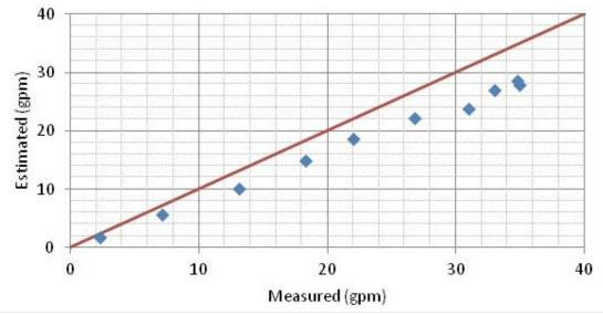
Figure 11: Measured VS Estimated discharge for flume C.
