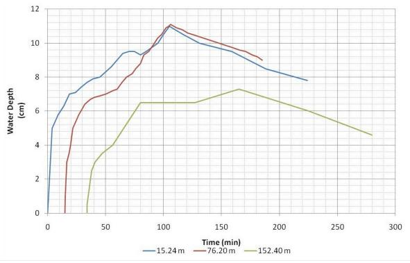
Figure 4: Hydrograph B2T2 at different locations along the border 2.
