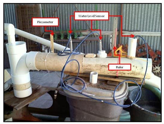
Figure 7: Location of sensors and ruler to compute flow rate over time.
