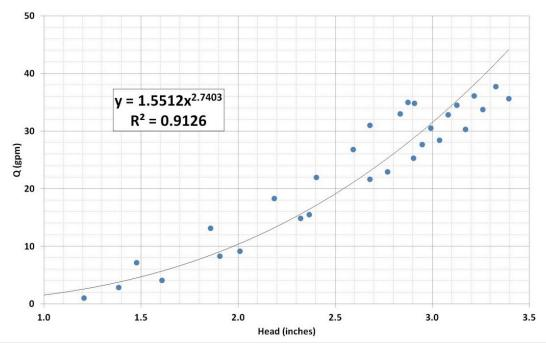
Figure 8: Circular Flume (Calibration)- Head-Discharge equation for a circular flume.
