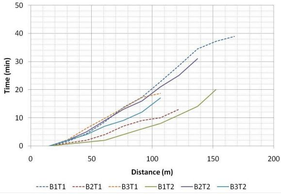
Figure 5 Advance curves for the six borders tested in the field.
