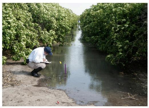
Figure 2 Water depth reading taken at the downstream end of the border.
