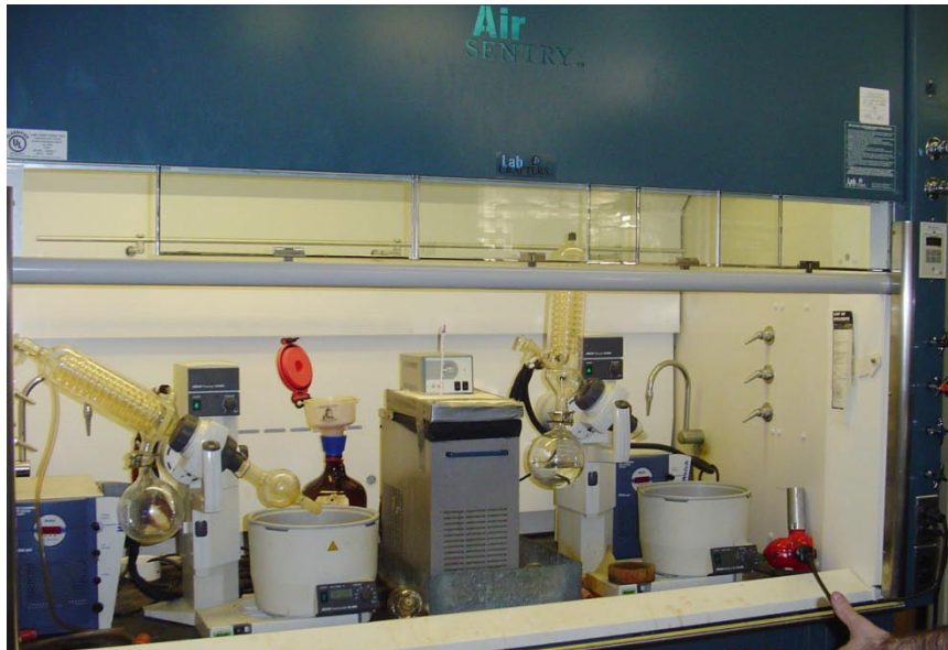
11 Figure 6. A Typical Hood System in a Lab
