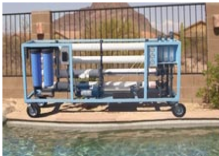
Figure 4. Pool Reverse Osmosis System
