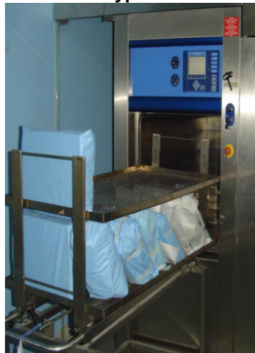
Figure 2 Sterilizer Being Loaded with Surgical Packs
