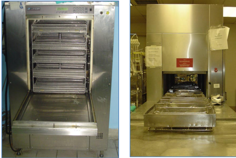
2 Figure 8. Batch and Conveyor (Tunnel) Washer - Disinfectors in Central Sterile
