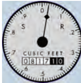
Figure A-1. Simple dial meter in cubic feet.
