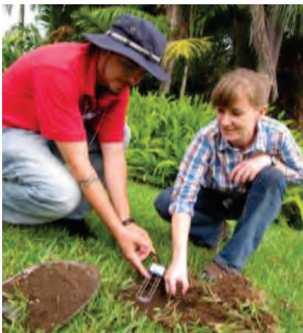
Figure 57. A demonstration of properly burying a soil moisture sensor.
