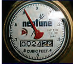
Figure A-3. Simple dial meter with turned over number.
